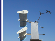
Eolo prototype, parallel configuration, operating in air.
