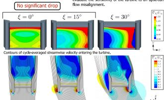
Contours of cycle-averaged streamwise velocity with streaklines in a plane at the mid height of the turbine
